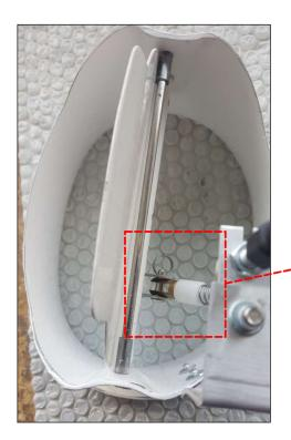
Attach the "Bowden cable" with the forked end to the "Cooler flap" using the "Splint pin" and the "Safety ring".
