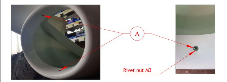
"Cooler flap" and "Lower engine cowling" after alignment, drill together according to position "A" first you must drill holes  $\emptyset$  3,5mm.
