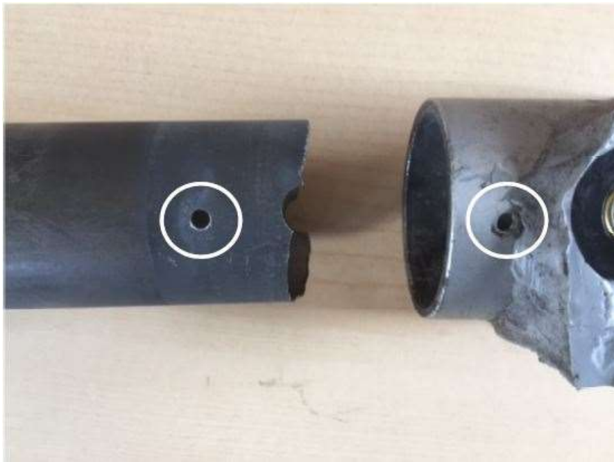
Figure 2: Failed A- pillar removed from outer sleeve part on right of picture. Circled holes show location of the rivet which was holding the parts together.
