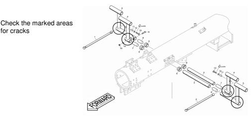
After carrying out the inspection, the pedal push-rods must be re-attached to the pedals and secured. The work may be carried out be a gualified person.
