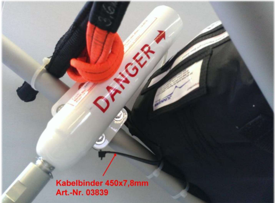
Figure 11: Securing the rescue container against sliding down
