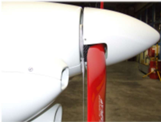
Figure 5: Attachment point between cowling and propeller spinner
