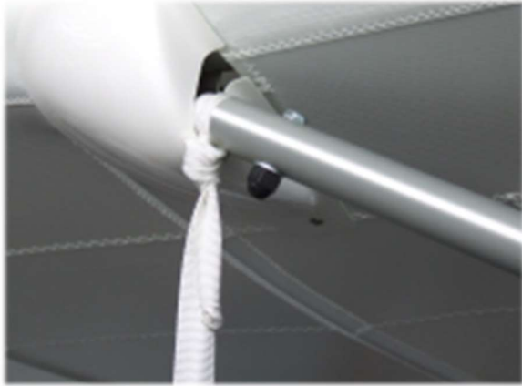
Figure 4: Upper attachment point on front lift strut
